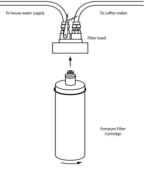
Electrolux ACCFILT-24 Filter Kit with Filter Installed
